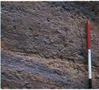
Detail of flood deposited sand, about 2 m down the trench wall. The water has eroded the small bluff (left). Dated by charcoal collected above and below the clean yellow sand, this flood occurred about 3200 years ago and is the highest recorded Murray flood.
